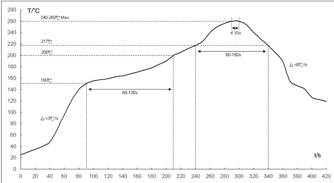
Fig1: Reflow soldering profile for lead-free solder (SnAgCu)
